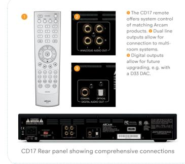
**Digital to Analogue** conversion 24-bit multilevel
